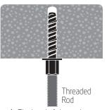
4 The head of the anchor should be set flush with the base material. Install the threaded rod. The thread should be fully engaged in the anchor.
