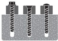
Continue to tighten the anchor until flanged head is firmly seated against fixture. Be sure not to over torque the anchor.
