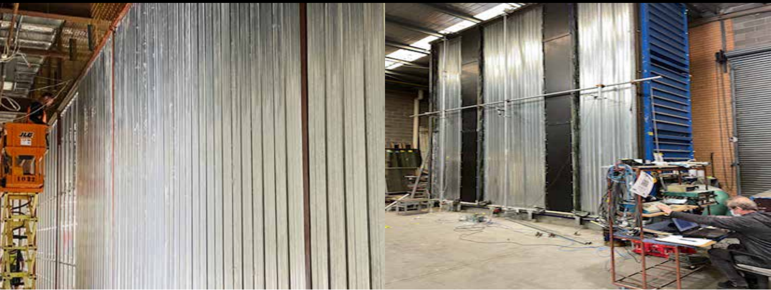
K8 SUPAPANEL® wind test being performed
